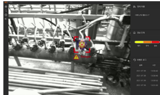
Leak detection monitoring system with AI 2 algorithm
