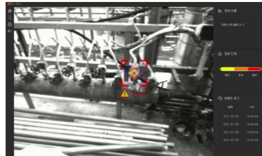
Leak detection monitoring system with AI 2 algorithm
