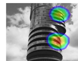
Building maintenance (Abnormal Noise Source)
